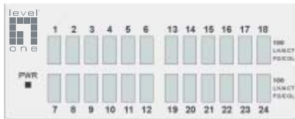
Figure 2-2 The LED Indicators
